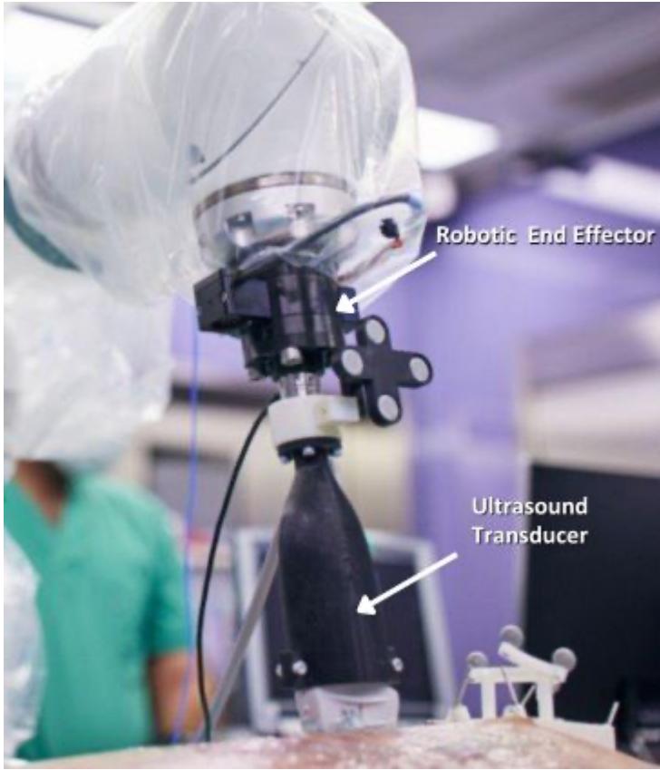
Figure 1: The FAROS robotic system with the robotic ultrasound end effector attached.
