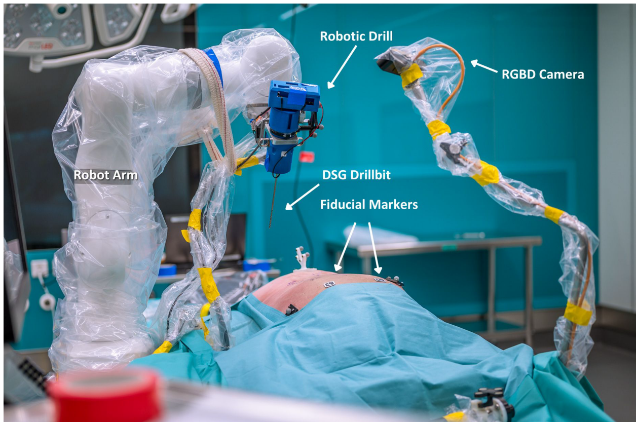
Figure 2: The FAROS robotic system with the robotic drill attached and fiducial markers placed for the optical (RGBD) camera.
